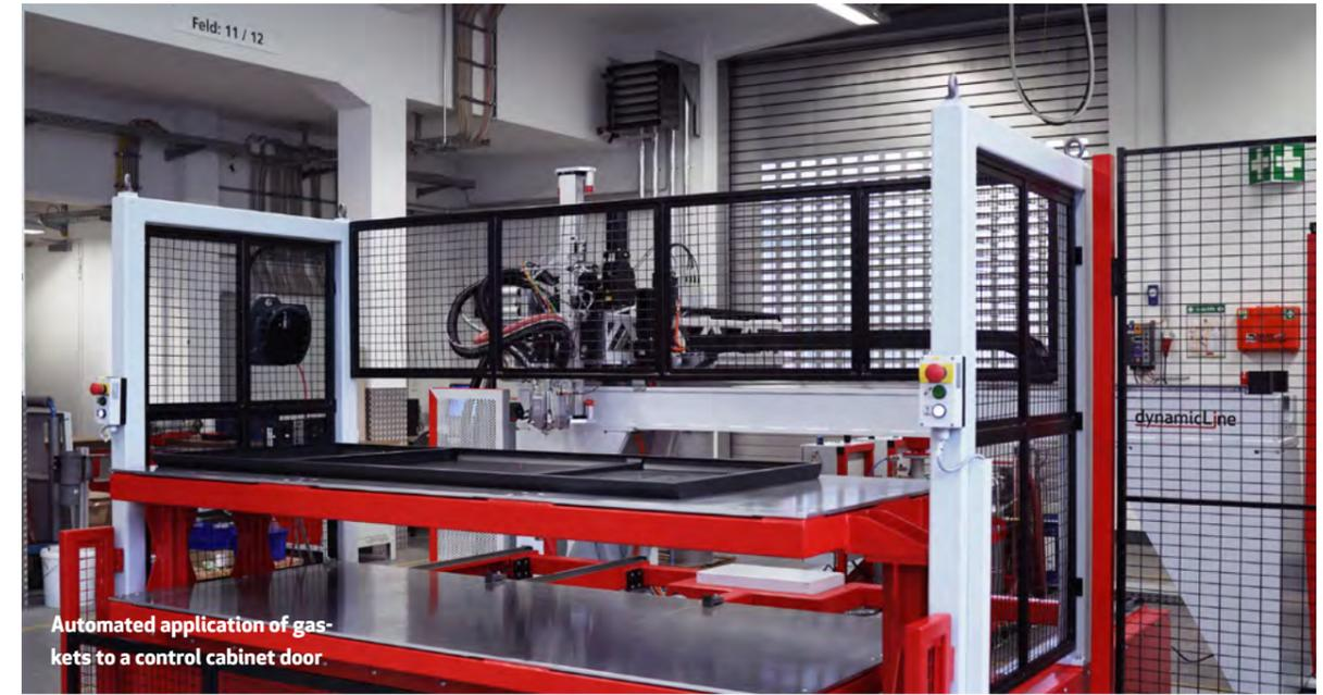
Automated application of gaskets to a control cabinet door.
