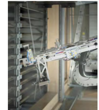
**Everything is fully automated in the production hall: the photovoltaic modules are bonded to the metal frame with the eldomix metering and mixing system. The material is supplied via gear pumps. They are then assembled into a complete retractable roof group.**
