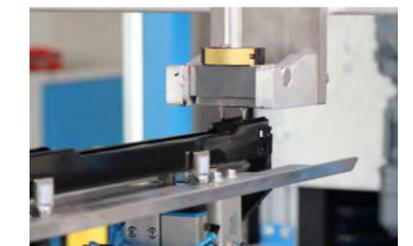
**Above: Automated application of adhesive to components for the production of oven doors. Pre-treatment with Pyrosil has already been carried out**
