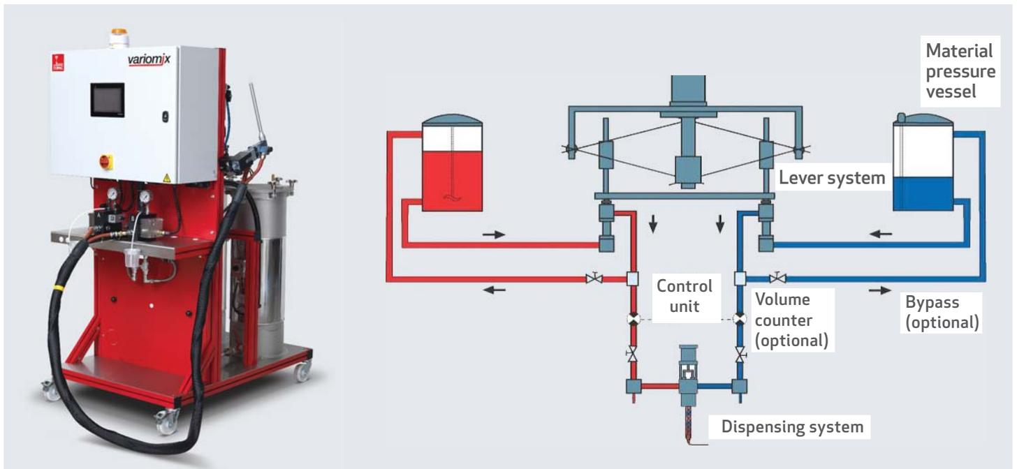
The variomix A is a pneumatic driven piston pump type metering and mixing system, used to handle low to high viscosity multi component media such as epoxy resins, polyurethanes or silicones. They can be unfilled, filled as well
