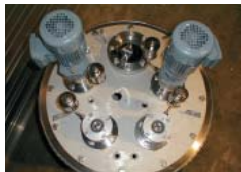
Special tank with two electric agitators
