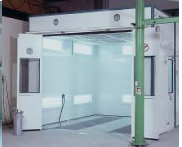
Combined spraying and drying booths
