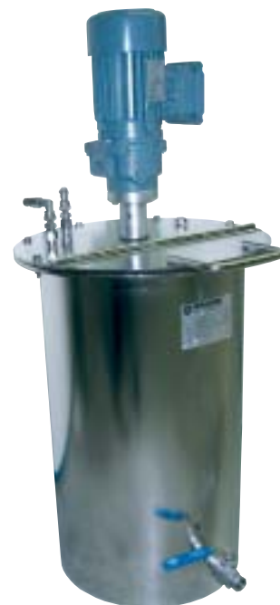
Mixing tank in electropolished design with electric agitator.
