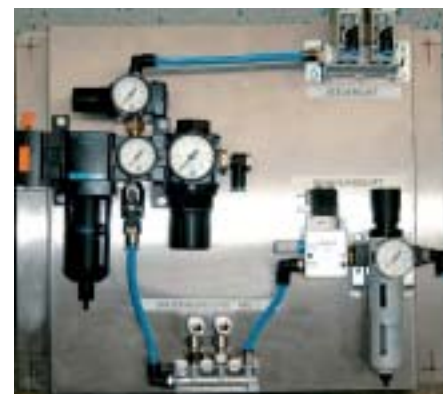
Control panel for arranging the compressed air supply units (instead of control cabinet)
