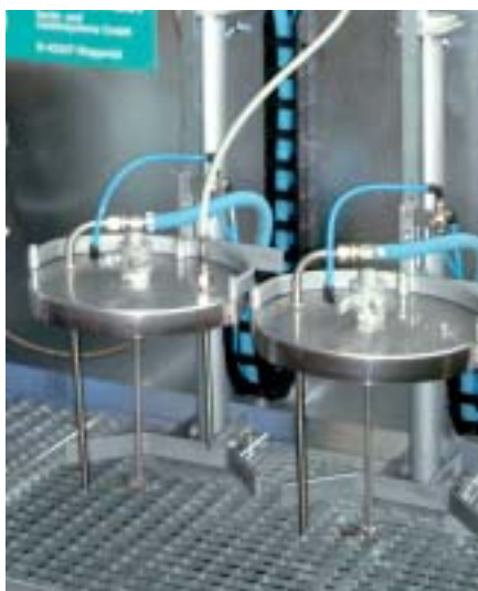
Installed lifts with covers and air-powered agitators for 30-litre drums.
