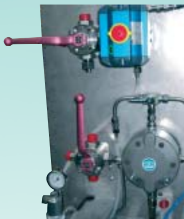
Installations for inserting and removing the pig for emptying and cleaning material pipes
