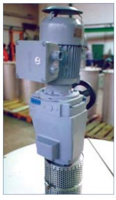
Electric adjustable-mechanism agitator
