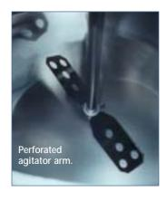
In this special container, the agitator motor and gearing are underneath the container base. The shaft and the agitator arm can therefore be easily removed.
