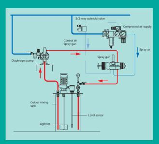
Type FMB paint tank with agitator, pump, compressed air valve, back-pressure regulator and level sensor
