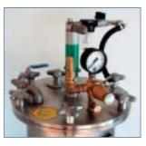
The new pneumatic agitator with a planetary gear is compact and powerful.
