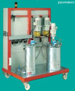
Machine for mixing and dosing two-component moulding materials such as epoxy resins, polyurethane, silicone, etc.
