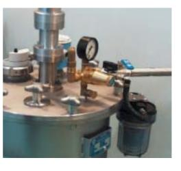
Pressure tank MDG 45 equipped with material filter and silicagel filter.
