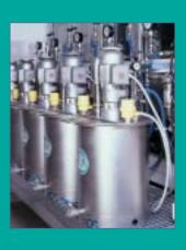
Rear view of a dosing and mixing system for moulded parts such as coils or heart
