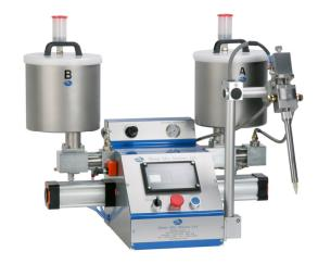
**Metering Pumps:** Single acting positive displacement.
