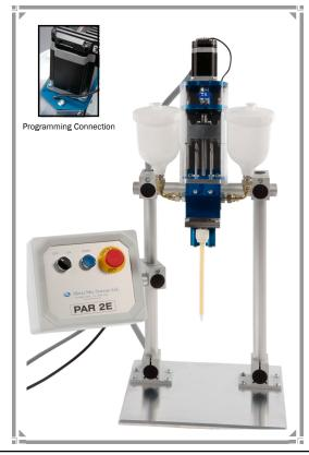
An extensive range of metering pump sizes and low volume disposable static mixing nozzles ensures that the PAR2-E can be tailored to suit most application requirements handling material mix ratios from 1:1 to 18:1.
