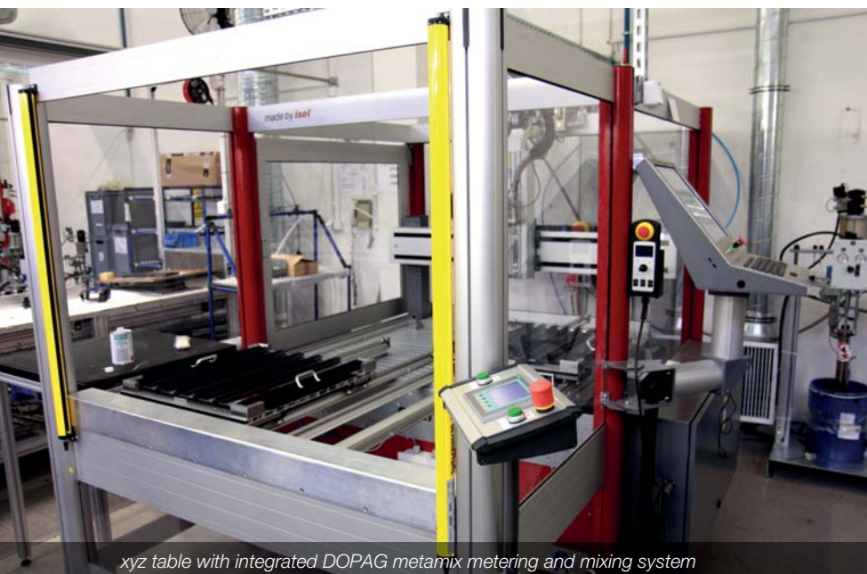
Dispensing of the adhesive beads with a 2K valve
