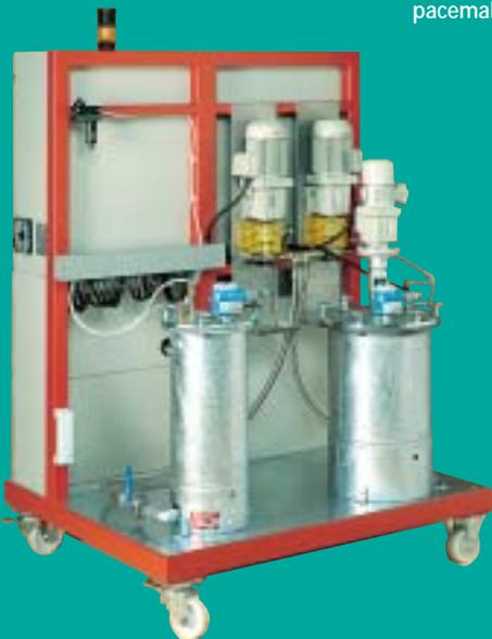
Machine for mixing and dosing two-component moulding materials such as epoxy resins, polyurethane, silicone, etc.
