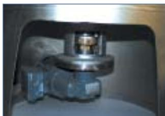
In this special container, the agitator motor and gearing are underneath the container base. The shaft and the agitator arm can therefore be easily removed.
