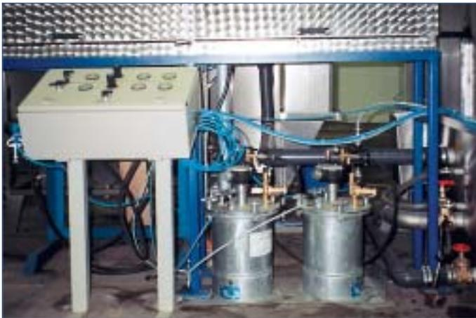
Pressure tanks and control cabinet for automatic application of separating agent for profiles
