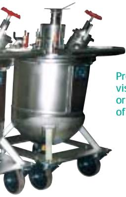
Pressure vessels for processing viscous masses (stone granulate or synthetic resin) for the manufacture of coils
