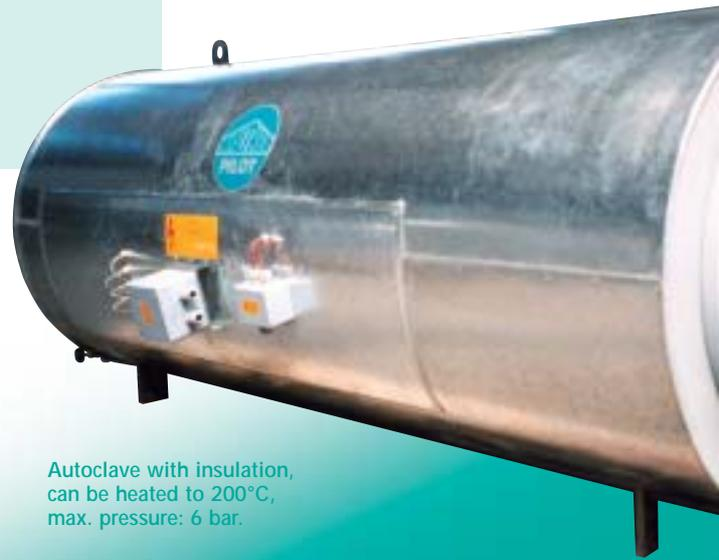
Autoclave with insulation, can be heated to 200°C, max. pressure: 6 bar.
