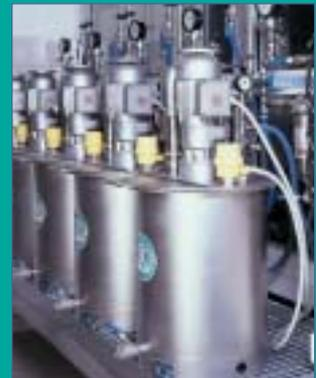
Rear view of a dosing and mixing system for moulded parts such as coils or heart pacemakers
