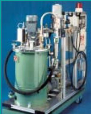
Colour dosing system for mass coloration of car steering wheels
