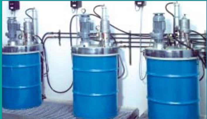
Barrel lids with lifters for material transport from the barrel
