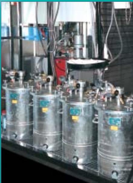
Two vacuum vessels as heating jacket tanks – 1000 litres and 500 litres – for polyurethane processing
