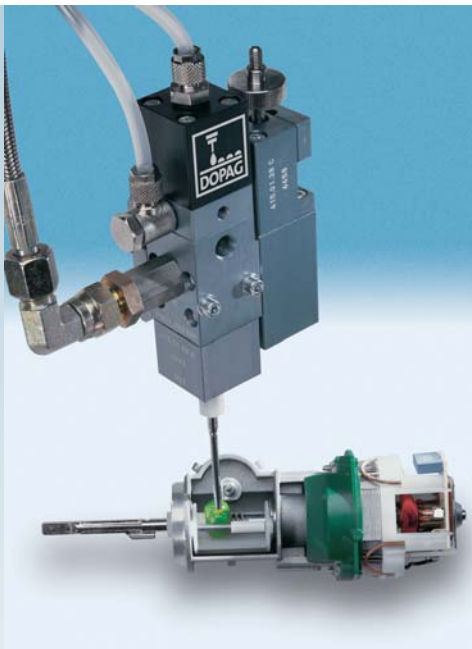
Lifetime lubrication of gears
