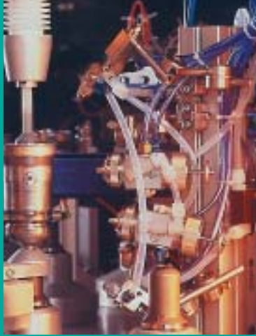
Coating airbag gas generators. Four spray guns aim at the conical workpiece. Coating rate: 3 - 4 seconds.
