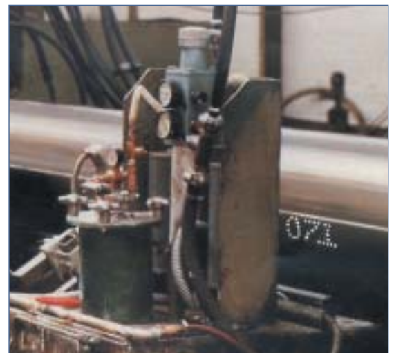
Marking of Pipes
